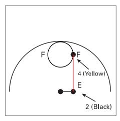
5. Place black ring at position "E". Bring yellow ring (4) to position "F" and make a mark inside yellow ring (4). Draw line from "F" to "E" along edge of string. Repeat this step for opposite side.
