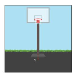
1. Mark a starting point(1) on the ground directly underneath center of backboard as shown
