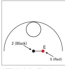
4. With black ring (2) under backboard, bring red ring (5) to position "E" and make a mark inside red ring.
