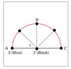
2. Have another person hold down black ring (2) on starting point mark. Bring blue ring (3) to position "A". Insert chalk into blue ring and draw line from position "A" to position "C". Note: String must be taught while drawing all lines.
