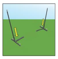
4. Install the lower black rods with coupling tubes up, into angled pipes.
