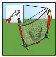
8. Hold black rod while pulling sleeve up. Loop white cord over rod top.
