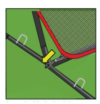
11. Take lower elastic loops and place under stud on both end legs. Wrap velcro around frame.
