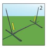
Install the two lower fiberglass poles, with coupling tubes at the top, into the angled pipes on the metal base.
