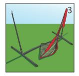
Thread a fiberglass pole through one of the net's sleeves making sure the net is right side up (white loops at the top corners and black bungees at the bottom corners).
