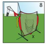
8. Grip the pole and slide the sleeve up before looping the white rope around the metal pole top.
