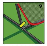
9. Loop the black elastic bungees over the metal posts located on the outside of each end leg. 10. Wrap the velcro around the frame (X in Fig. 8).
