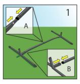
Join the two slightly bent pipes together (Fig. A)
