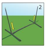
2. Install the two lower fiberglass poles, with coupling tubes at the top, into the angled pipes on the metal base.
