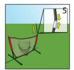
Insert an upper fiberglass pole into one of the lower pole's coupling tube. The metal knob should be at the top.
