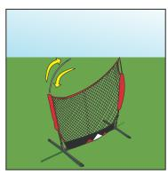
4. Pull the other fiberglass rod inward to thread the other sleeve over it. Then attach the white cord.
