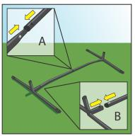
Join the two slightly bent pipes together (Fig. A)
