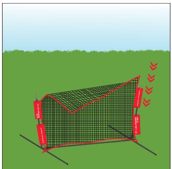
**4)** Thread the sleeves over the poles making sure that the black bungees and Velcro straps are on the bottom.
