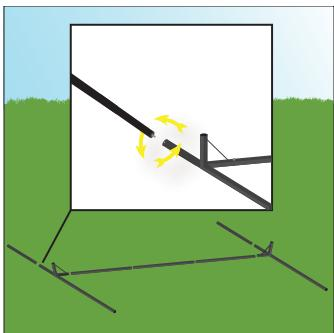
**1)** Screw the leg extenders onto the legs.
