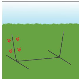
**3)** Insert the two bottom fiberglass rods (with coupling tubes on top) into the base.
