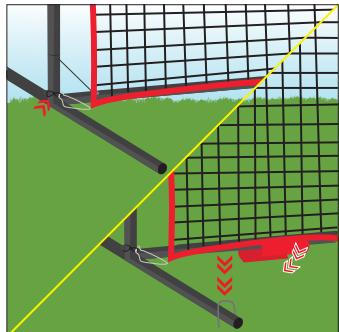
**7)** Attach the black bungees at the bottom of the net to the metal posts on the outside of the legs. Then wrap the velcro straps around the base bar. The stakes will help in windy conditions.
