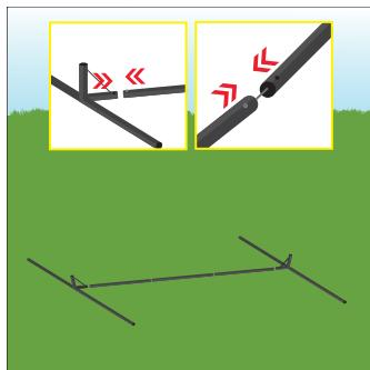
**2)** The base bars are connected by cables. Use the buttons to snap them together. Then attach them to the legs.
