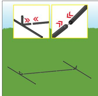
**1)** The base bars are connected by cables. Use the buttons to snap them together. Then attach them to the legs.
