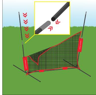
**4)** Insert the upper fiberglass rods into the metal coupling tubes of the bottom rods.
