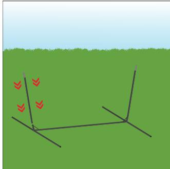
**2)** Insert the two bottom fiberglass rods (with coupling tubes on top) into the base.
