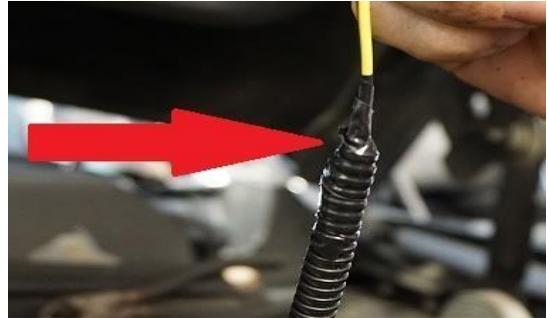
12. Place the wire loom and wires to the side.
