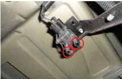
**3.** The UREA injector is located between the CAT and DPF, above the torsion bar crossmember. Unplug the electrical harness and the UREA line from this injector. The injector can remain in the factory exhaust and be removed from the truck if installing a downpipe-back exhaust system. Leave unplugged injector bolted to factory exhaust if only installing a cat-back exhaust system. The wiring harness and urea line may also be removed from the truck, or zip tied out of the way.
