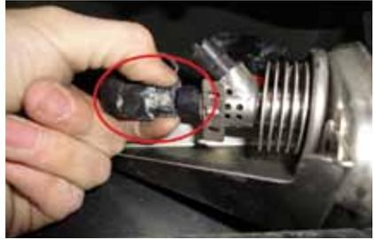
**4.** The main UREA harness MUST be unplugged. The main UREA harness is the large black harness located near the UREA injector and above the UREA fluid tank. Flip the large gray locking tab to disconnect the harness. At this point you may also remove the entire UREA tank from the truck. This is recommended but NOT necessary.
