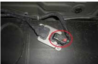
6. In order to shut down the EGR process completely on your LML, you must unplug 3 harnesses under the hood. See pictures for locations.
