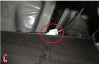
**2. The DPF pressure sensor is located under the bed in front of the axle on the inside of the passenger side frame rail. Pull the rubber lines from the sensor. These lines may be removed along with the DPF, but leave the electrical harness plugged in to this sensor.**
