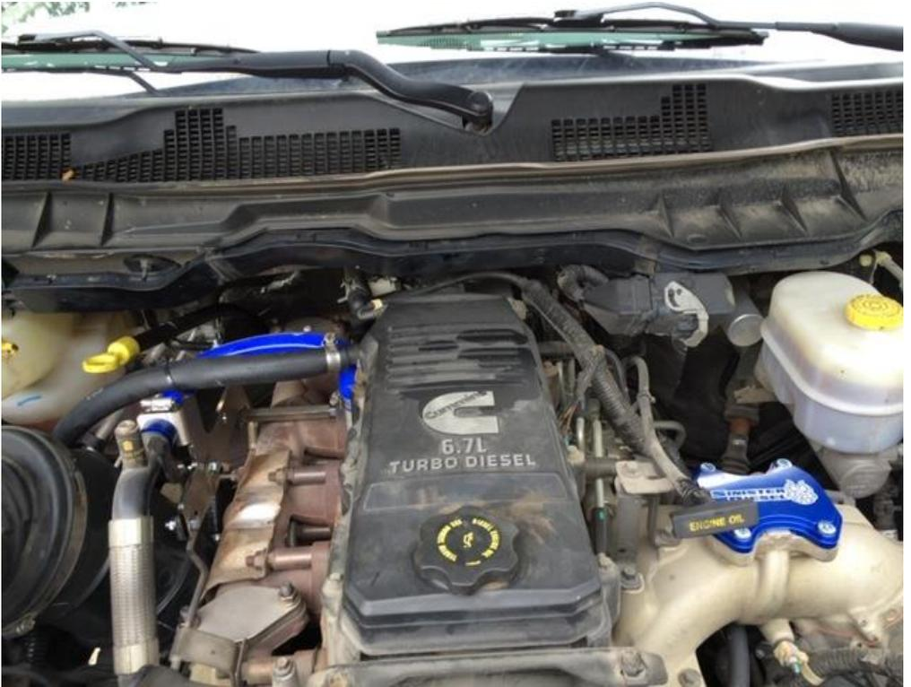
The Exhaust break sensor (EBP) with the brown plug can be clocked back toward the fire wall and reattached to the back bolt of the egr delete mounting kit. Depending on which egr delete kit you purchased you can also just reposition the (EBP) sensor to where ever you want and drill a new attach hole in the main mounting bracking.
