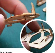
Cut the ply parts from the surrounding material and slot 2 x W4 into the two edges of W3 as shown above. **NB:** ensure W3 text is facing upwards when attaching W4.
