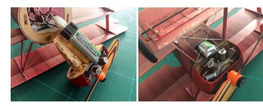
Connect the battery to the receiver and place on the battery plate on the motor mount.
