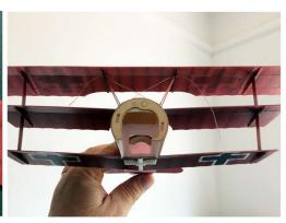
Before assembly of the upper wing partially release the tip of the aileron to allow some washout to be introduced into it if required during trimming of the aircraft.
