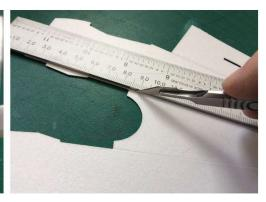
Using a sharp craft knife, remove the slotted areas from D1 and D2 as shown above. This makes room for batteries larger than 80mAh to fit into the fuselage.
