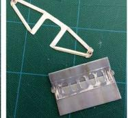
Remove Undercarriage parts P16, P17 & P18 from the plastics sprue. Attach P18 & 17 to the unprinted side of P16 as shown in illustrations above.
