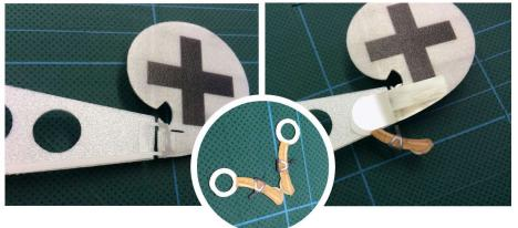
Attach plastic hinge joint P2a to the rudder Z2 on the port (left) side as shown in the above image. Then attach the other half of P2a to the port side of the airframe at the rear. Ensure there is ~1mm gap between the rudder and the frame.
