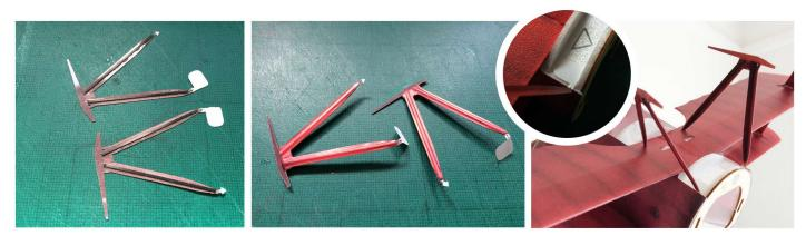
Attach 4 x 41mm of 0.4mm x 1.0mm carbon fibre strip to each leg of P13 & P14. (Cabane struts)
