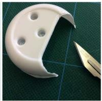
Gather the parts that are used to create the cowl. This includes the vac formed plastic, the laser cut plywood sheet and a 4mm x 1mm neodymium magnet.
