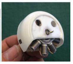
Slot and glue the motor mount assembly into the back of the firewall assembly as shown above.
