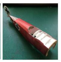
Carefully apply glue to one side at a time and work around the fuselage until the airframe is wrapped with Z1.
