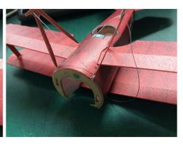
Using the guide at the front of this manual, sand and score Z9 before applying it to the deck area in front of the cockpit. Once scored, pre-bend Z9 to assist with the fitting.
