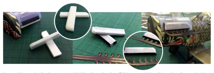
Assemble a pair of exhaust port shielding from the four D31 parts sticking 2 together for each side. Sand a curve on one long and one short edge on each structure. NB. Ensure that each is sanded as a mirror image of the other.
