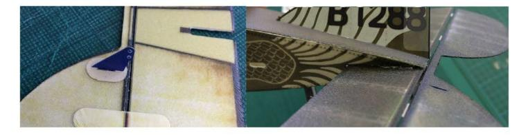
Slot P9 into P8 to create the elevator control horn. Attach horn to the underside of the elevator in the pre-cut slot provides.
