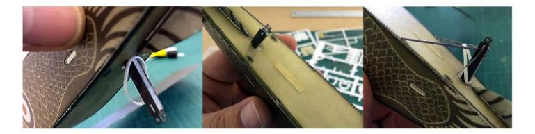
Attach the white elastic to the tail skid main strut as shown in the image. Attach S26 to the exposed Depron on the underside of the fuselage.
