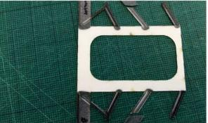
Add 2 x 35mm strips of 0.4mm x 1.0mm carbon fibre to the leading edge of the undercarriage part P13. Glue parts P14 - P17 to the back of P13.
