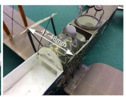
Attach parts P40 & P43 to the unprinted side of cabane struts part P38.
