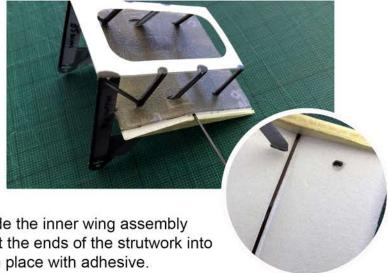
Fold undercarriage assembly as shown. Slide the inner wing assembly from the rear of the undercarriage and insert the ends of the strutwork into the holes provided in the wing and secure in place with adhesive. (Super'phatic glue is useful here).
