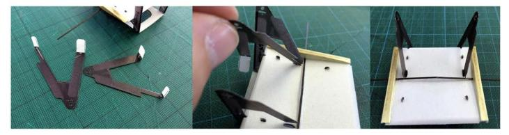
Fold the ends of parts P18 and attach to the main undercarriage by sliding the rear most leg through the centre hole in the inner wing. Repeat the process with P19 on the opposite undercariage leg.
