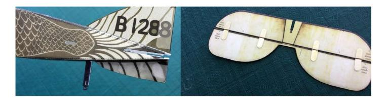
Attach Z6 (Top vertical stabilizer) and Z8 bottom vertical stabilizer) to fuselage in slots provided. Ensure both are perfectly verticle. Once in place it's advisable to run either a thin line of Super'phatic or CA either side of the join with the fuselage to stiffen the joint.
