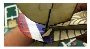
Attach S5 & S6 (hinges) to the port side of the vertical stabilisers above & below the fuselage. There are shaded areas on these parts to show the location of the stickers.
