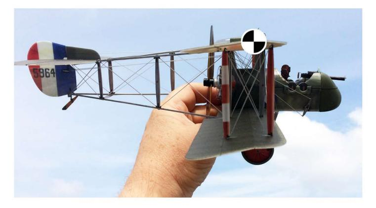
With battery installed, the Centre of Gravity should be located on the crease of the top wing.
