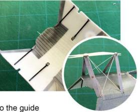
Prepare fuselage skin Z2 by scoring and beveling according to the guide provided in these instructions.
