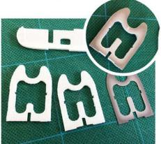
Attach 2 x P1 to either side of D1 at the nose and along the lower edge of the Depron foam part to create the keel.
