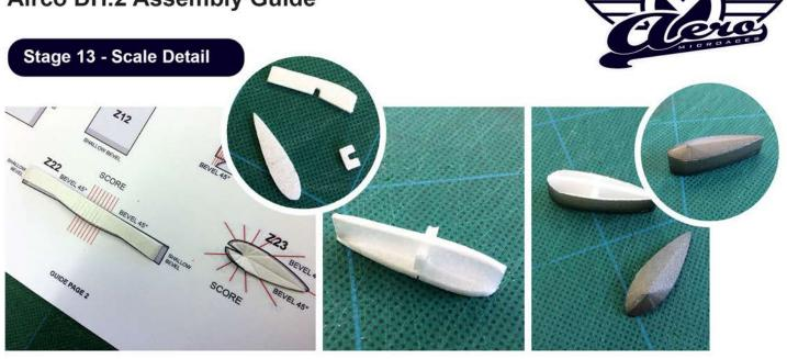
To create the emergency gravity fuel tank score and bevel Z22 and Z23 according to the guide.
