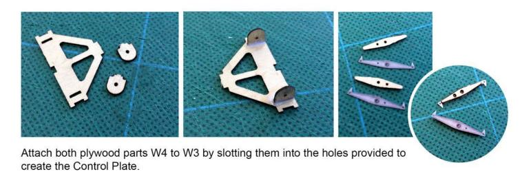
It's recommended that aliphatic resin is used to bond plywood to plywood.
