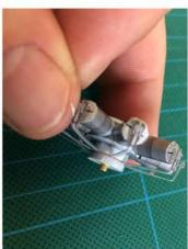
Fold the ends of the con rod part P27 at right angles. Install P27 onto the front of the engine assembly and secure. Slot the protruding parts of each cylinder through the slots in the ends of the rods on P27. Secure each rod end in place with a drop of CA or aliphatic resin.
