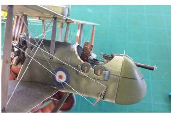
Cut the profile pilot figure supplied, fold and glue the two halves together.
