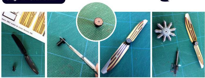
The recommended prop for the Microaces Airco DH.2 is the GWS4530R reverse pitch prop. This provides the correct direction of thrust with the motor turning in the direction it was designed to. **NOTE:** Using a normal pitch prop and running the motor in reverse may severely shorten the life of the motor.
