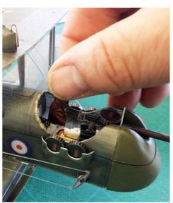
The recommended battery for the Airco DH.2 is a 100mAh or 130mAh Lipo.
