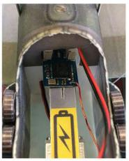
The recommended receiver for the Airco DH.2 is the Microaces Plug and Play Micro 4-7 channel receiver pictured above.
