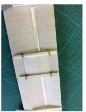
Attach the shorter ribs to the centre rib positions marked on the upper wing parts Z13 & Z14 ensuring that the pale side of the stickers wrapped around them face outwards.
