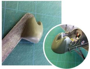
Paint the supplied polystyrene vac formed nose. The suggested colour is a mix of Matt Ocean Grey and Matt Khaki Drab in ratio of 4:1 grey to green. Enamel or acrylic paint can be used.
