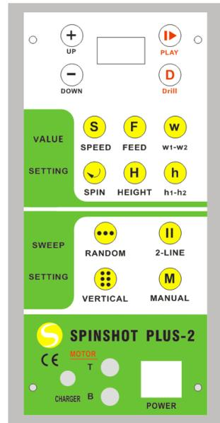
**If anytime the machine functions improperly, the user can turn off the power button to reset machine’s control logic. Most of the time, the improper working of the machine is caused by low battery voltage.**
