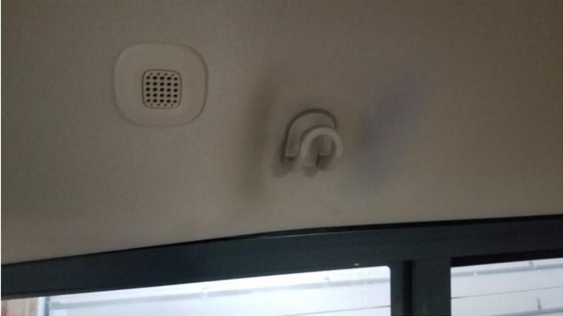
With everything removed, you can carefully fold back the rubber seal at the door and work the headliner down. The back of the headliner just sits on the black molding above the window.
