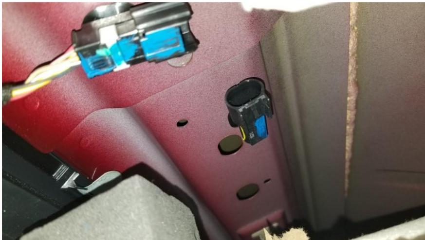
The right hand connector is actually a terminator that tells the CAN C buss that it doesn't have an open circuit. You need to pull this part out of the mounting hole. It will not be used.
