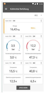
Added refrigerant is displayed in g/kg increments on the manifold/app.
