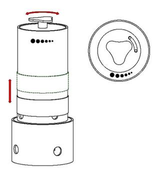
If your water level is too low you may hear a "water crashing" noise. To minimize the water crashing noise lower the Silencer Sleeve and readjust reactor.
