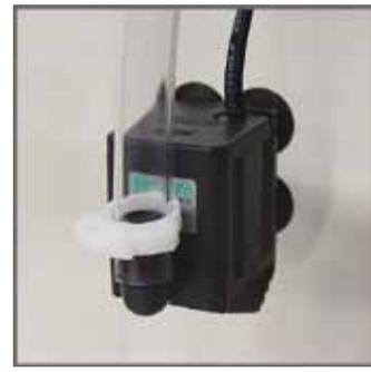
3. Attach clear PVC u-bend barb fitting to end of cut tubing. Attach other end of tubing to pump. Secure with hose clamps.
