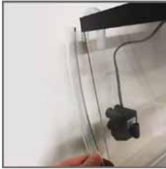
2. Determine pump location and cut a piece of tubing to appropriate length.
