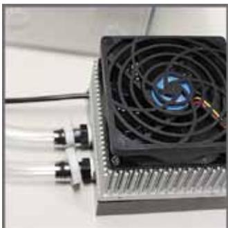
7. Tubing should now be connected to chiller as shown.
