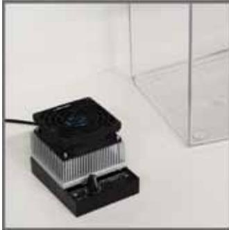
1. Place chiller in desired location ensuring adequate space for air movement.
