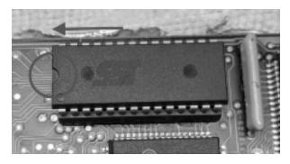
6. Once your new RK-Tunes chip has been installed you can close the ECU and reinstall ECU into the vehicle.
