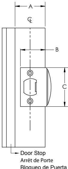
Dimension B & C should be used as reference only. Due to tolerances as reference only. Due to tolerances actual door jamb prep dimensions will vary. Using the strike plate outline edges and locate screw holes on strike with center line on jamb.
