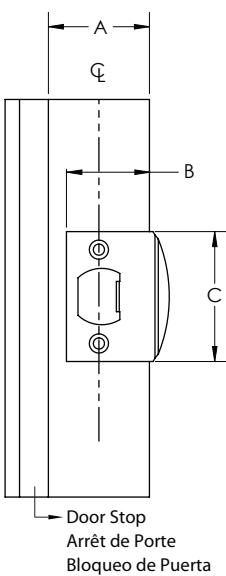
Dimension B & C should be used as reference only. Due to tolerances as reference only. Due to tolerances actual door jamb prep dimensions will vary. Using the strike plate outline edges and locate screw holes on strike with center line on jamb.
