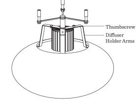
4. Settle Diffuser on Diffuser Holder so that the Arms grip the inside lip of Diffuser. Gently lower Shade.
