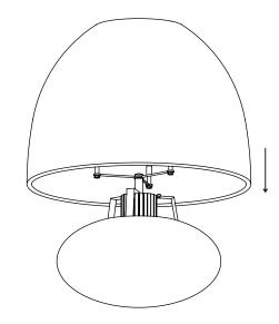
5. For future removal, reverse Steps 2–4, with the light turned off. Clean with a soft damp cloth and non-abrasive cleaner.
