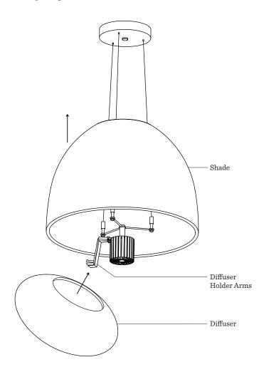
3. Hold Diffuser level and locate the brass Thumbscrew on the Diffuser Holder. Grasp the Thumbscrew to fan out Diffuser Holder Arms until they are evenly spaced and stop in place.
