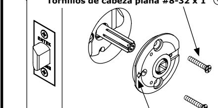
**Step 3: A.** Fully extend spindle by pulling it outwards until it is against the internal stop. **B.** Tighten the pre-installed set screw in knob or lever with 3/32" Allen Wrench ⑭.
