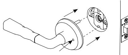
**MAKE SURE THE RELEASE HOLE LINES UP WITH THE PRIVACY PIN ON THE INSIDE.**
