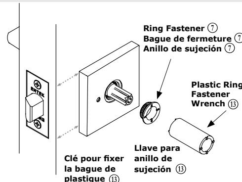
**Check trim alignment before fully tightening Ring Fastener.**
