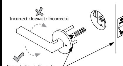
**⚠ Make sure the release hole is close to door edge (applicable only to privacy function).**
