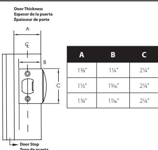
**NOTE:** Dimensions B & C should be used as reference only. Due to tolerances actual door jamb prep dimensions will vary. Using the strike plate outline edges and locate screw holes on strike with center line on jamb.
