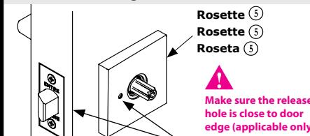
**⚠ Make sure the release hole is close to door edge (applicable only to privacy function).**
