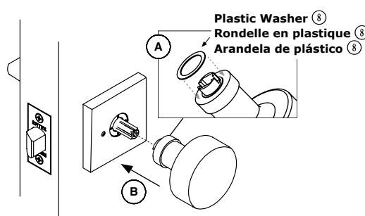
**Step 7: A. Place Plastic Washer ⑧ on to Knob or Lever ⑨. B. Then install Knob or Lever ⑨ by sliding it on to the spindle.**
