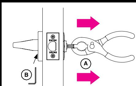
**Step 4:** Insert short end of 3/32" Allen Wrench ⑭ into spindle as indicated and **tighten approximately one full rotation**.
