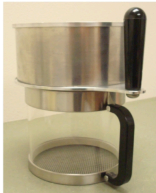
Completed roast chamber/chaff collector assembly.
