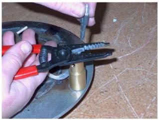
Cut old connectors from RTD, this will allow the RTD to be removed from the spacer.
