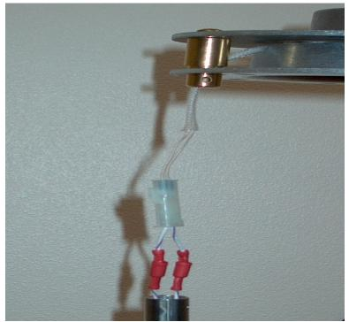
Install the new Assembly as shown ensure that connector locks, and then slide the connectors down the tube until the smoke box sits flush with tubes.
