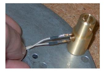
Insert RTD wires into the spacer hole and feed through. Ensure that the pins are not damaged in the process.
