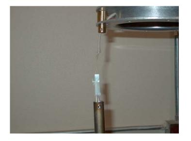
The new style connector does not require the adaptor. Ensure that the connector locks before inserting into tube.
