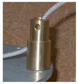
Ensure that the braided sleeve is passed through the spacer.
