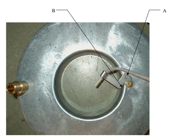
If the connectors are the old style, the supplied adaptor must be installed. Insert the connector and press firmly until fully seated.
