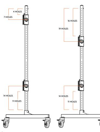
Install top and bottom brackets using screws J and I.
