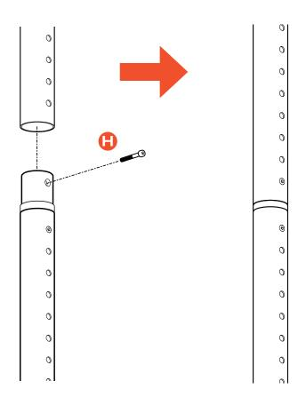
Secure Boot Bracket to each Pole Upright. To do so, attach the bracket on the side of the pole that is marked with the J label. Use Screw K to attach each Boot Bracket as shown.
