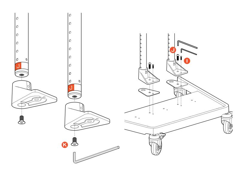
Install Slider Mounts to Pole Uprights and adjust to the desired heights.
