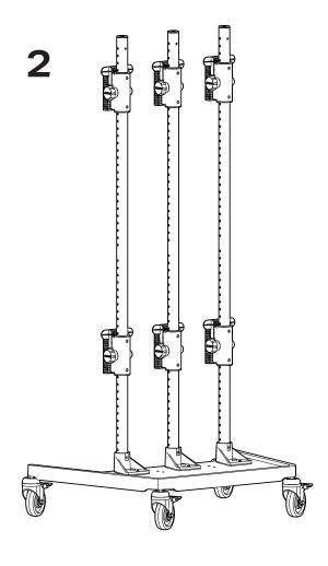
Install top and bottom brackets using screws I and J.
