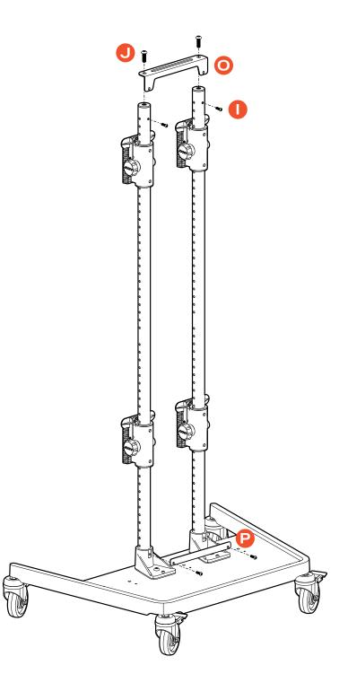
To adjust the Slider Mount, turn the knob counterclockwise ~1 turn and pull out. Slide the mount up or down based on your desired height. To secure the Slider Mount tighten the knob by turning it clockwise until hand tight.
