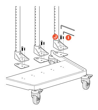
Install Slider Mounts to Pole Uprights and adjust to the desired height.
