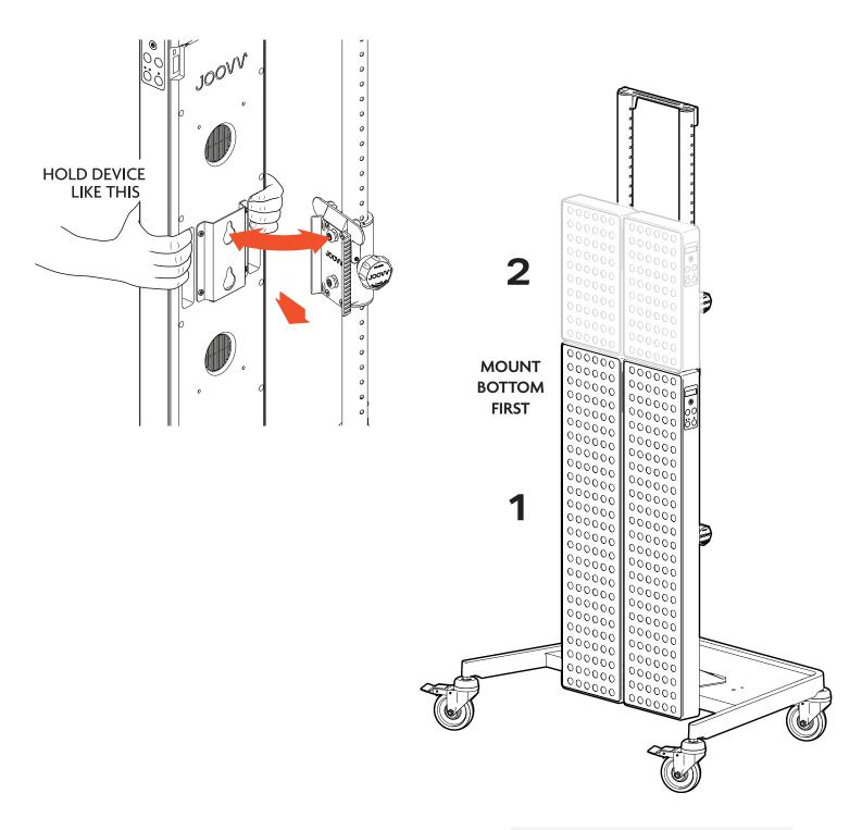
To remove the Solo or Mini Device from the Slider Mount, follow the steps illustrated below.
