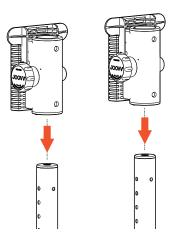
FOR QUAD CONFIGURATION, SLIDE THE TOP MOUNTS ONTO THE POLE UPRIGHT SO (4) HOLES ARE SHOWING ABOVE THE MOUNTS
