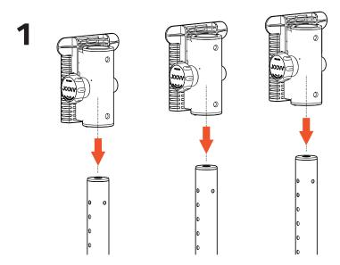
FOR ELITE CONFIGURATION, SLIDE THE TOP MOUNTS ONTO THE POLE UPRIGHTS SO (4) HOLES ARE SHOWING ABOVE THE MOUNTS
