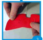
Align the holes and edges of the reinforcement piece with the prepunched holes and edges of the sail.
