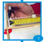
The Bottom Tensioning line is marked at 3 3/4".
