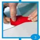
Carefully align the holes and edges of the Corner tab Set with the prepunched holes and edges of the Sail.
