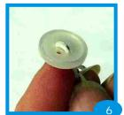
Use the Wire Loop to thread the loose end of the Tensioning line through two diagonal holes of the Button.
