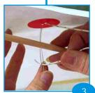
Push the Wire Loop through the second hole from the front of the Sail
