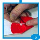
With the Spine in the pocket, slide the square end down towards Sail. Pull the zip tie just tight enough to hold the Spine in place. But, not so tight that you can't take the Spine out.
