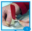
Start with one of the Corner tab sets. Match it to a corner of the Sail to make sure you have the correct orientation before you do the next step.
