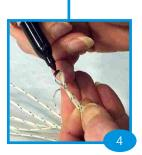
Use a permanent marker to mark the center of the Bridle line.
