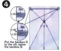
Fix the bamboo D with scotch tape. Attach the bamboo B to the upper side of the double-sided tape.
