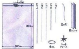
Materials Sail (Japanese paper) lpc (288mm long) Bamboo A 2pcs Bamboo B (272mm long) 1pc Bamboo C (255mm long) 1pc Bamboo D (172mm long) 2pcs Bamboo E (110mm long) 1pc Connector 1pc Tail 2pcs Bow line 1pc Rubber band 2pcs
