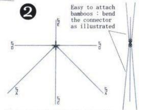
Insert the bamboos to the connector as shown above.
