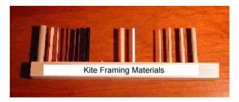
**Suggestion:** Make a display of kite framing materials. Drill holes into a long strip of wood and insert examples of different frame materials such as bamboo, fiberglass, carbon fiber, and wooden dowels. Examples should include solid and hollow rods.
