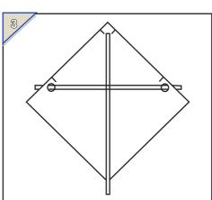
Pass the horizontal spar through the holes and attach it with glue. (Do not attach the bark side of the bamboo)
