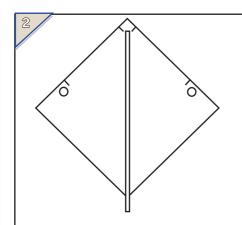
Attach the vertical spar to the paper with glue as illustrated. (Attach the bark side of the bamboo)
