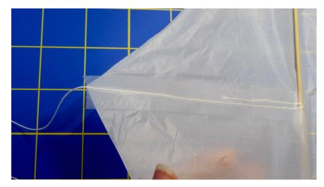
Tape this line down, from the spar out to the wing tip.
