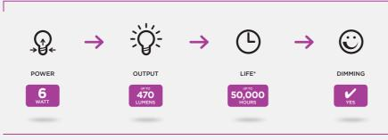
\* We test our lamps to both L70 and L90 standards. Figure shown is for L70. Operating temperature -30°C to +40°C
