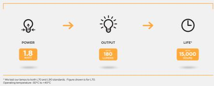
Megaman's latest G4 LED lamp is now even smaller, which means it is now suitable for even
