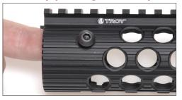
2. Loosen the three screws by two full turns with 5/32 allen wrench.
