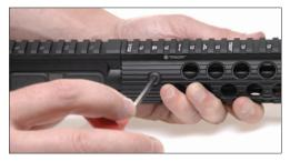
4. Holding rail into position, tighten the three retaining clamp screws evenly. (For best results use thread locking compound.)
