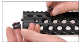
\*If screw comes out of clamp, make sure tapered end is facing end of rail and nut lip is in groove of rail.
