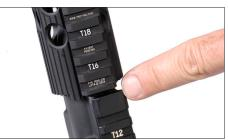
3. Slide rail onto barrel nut while rotating rail 5 degrees "clockwise" until flush with receiver, then rotate back to align rail with upper receiver.
