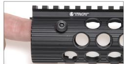
2. Loosen the three screws by two full turns with 5/32 allen wrench.
