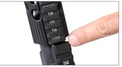
3. Slide rail onto barrel nut while rotating rail 5 degrees "clockwise" until flush with receiver, then rotate back to align rail with upper receiver.
