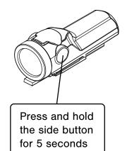
Top LED indicator will flash blue when pairing mode is enabled.
