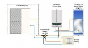
A special manifold is installed to connect the Audax heat pump and the boiler. The Audax is the primary heat source and the boiler will operate only when it is not economic to run the heat pump, or when there is a very high heat demand in the system. The boiler carries out the domestic water heating.
