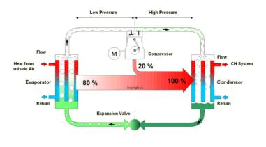
An Immergas Audax heat pump uses an electric motor to pump a refrigerant gas through an evaporator and condenser. The refrigerant gas acts as the heating medium.
