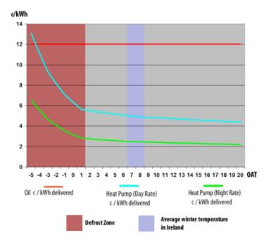
The graph above shows the typical costs of running an air to water heat pump versus an oil boiler. The cost in cents per kWh delivered is shown on the side and the outside air temperature is shown across the bottom.
