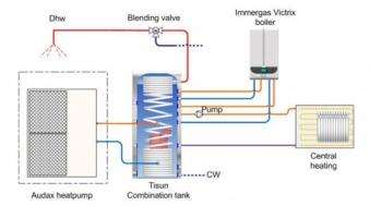
This system also allows the use of a special "night rate heat boost" function. The night rate heat boost function allows heat, produced by the heat pump on low-cost night rate electricity, to be stored in the combination heat tank. The heat produced using night rate electricity can cost as little as 2 cents per kWh. Typically, the additional cost of choosing a combination tank type system can be paid back in under two years when using the night rate heat boost function.
