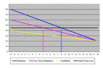
On Standard Radiators, we can see that at outside air temperatures above approx 8 degrees the heat pump can supply the required temperature economically.
