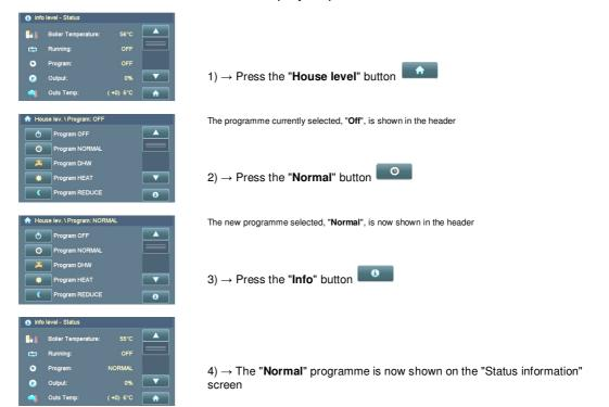
After activating the "NORMAL" heating programme, check the selected programme on the "Status information" screen. As soon as heat is called for and there is sufficient heat in the thermal store, the heating circuits start up fully automatically.
