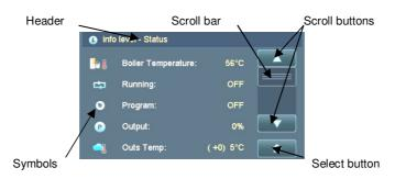
The header contains information about the level or menu selected. Operating statuses, sensor readings and switch conditions can be queried in the Selection window. The various buttons can be used to change and save settings or switch to different levels or menus, for example. You switch between the levels and menus by touching the buttons directly on the display screen.
