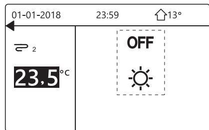
Use the control panel to switch the DHW unit on or off. Press “▶” and “▼” on the home page, the black cursor will appear:
