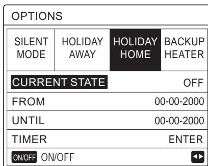
Use the “ON/OFF” key to select activated (ON) or deactivated (OFF) and use “◀”, “▶”, “▼”, “▲” to scroll and adjust.
