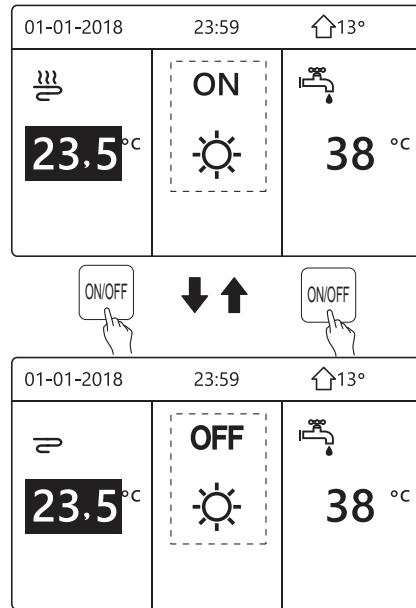
Use the room thermostat to switch space heating or cooling on or off.
