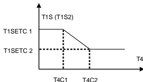
State: in the setting of the control panel, if  $T4C2 < T4C1$ , exchange their value; if  $T1SETC1 < T1SETC2$ , exchange their value
