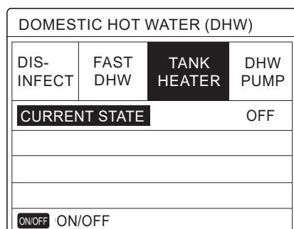
Use the “ON/OFF” key to select activated (ON) or deactivated (OFF). Use “BACK” to exit.
