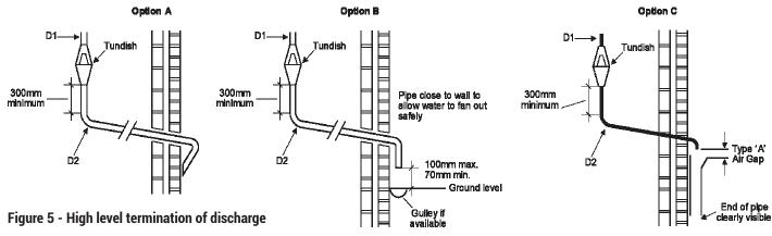
At high level, discharge onto a roof is acceptable providing the roof is capable of withstanding high temperatures and there is a distance of 3 m from any plastic guttering systems that would collect such discharge.
