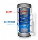
The Proclean tank is like a large central heating buffer tank. This means that it is full of the treated central heating water (CH Water) that circulates around your radiators and through the central heating side of your boiler.
