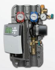
The FlowSol® B/BHE is equipped with an insulation casing featuring an innovative hinged controller panel, allowing for quick and easy access to the hydraulic components without dismounting the controller.
