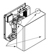
Installation requires no. 4 screws Ø 8mm (not included), suitable for the type of wall. The position must be selected to allow easy connection of the pipes to the appliance.
