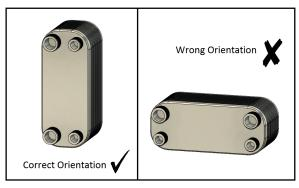
Install the heat exchanger so that the water from the stove can move upwards through it as shown. Do not install it horizontally.
