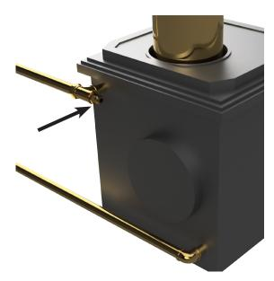
Install the sensor of the VST100 thermal safety valve as close to the stove as possible. A tee may be installed as shown in the image. The sensor is fitted in a 150mm immersion pocket which has a G 1/2 thread.
