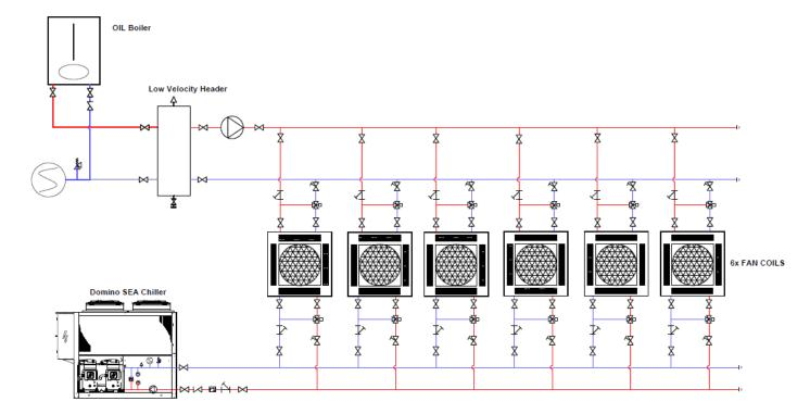
The chiller has an inverter-driven, speed-controlled pump that operates in constant pressure mode to deliver the required flow rate of chilled water to the system.
