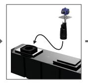
Insert the pump assembly into the tank via the top mounting hole
