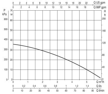
Based on kinematic viscosity values = 1 mm²/sec and density equivalent to 1000 kg/m³. Curve tolerance according to ISO 9906.
