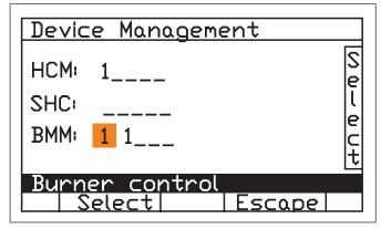
The display shows the status and the active sections of the system: ( inactive / 1 active)
