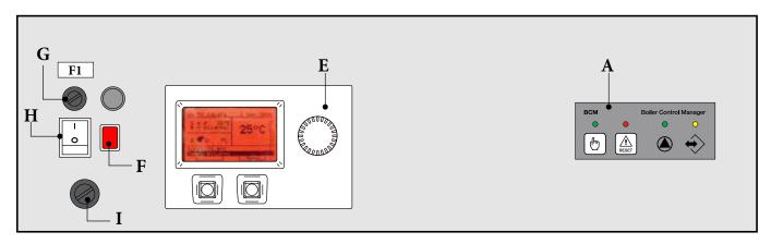
The BCM board prevents the system from shutting down if management of the HSCP system or main boiler system are out of service (see the BCM manual).
