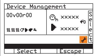
with knob "C" and press key "A" in order to access the technical programming area of each device (you must enter password 0000).
