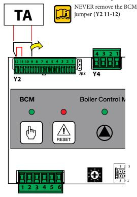
Set up on the terminal board, BCM (Y2 9-12) Remove **only** the jumper BCM (Y2 9-12)
