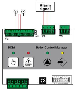
Connect the cables as indicated (Y4 3-4) Connect the cables (Y4 7-8)
