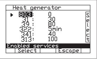
Select the parameter using knob "C". Press "A" (selec).
