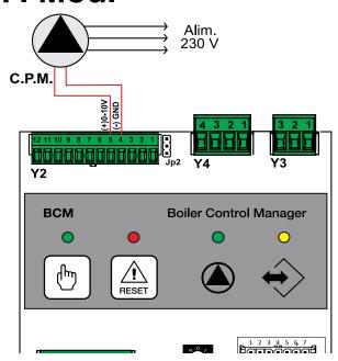
Connect the modulation control cables as indicated (Y2 4-5). External power supply 230 V-50 Hz.
