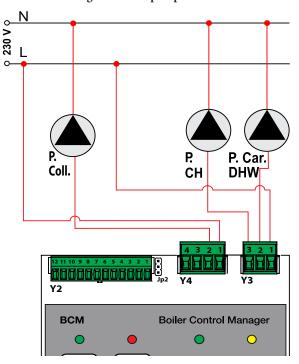
Connect the cables as indicated (Y4 1-2) Connect the cables as indicated (Y3 1-2-3)
