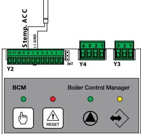
Connect the temperature sensor cables as indicated (Y2 6-8).
