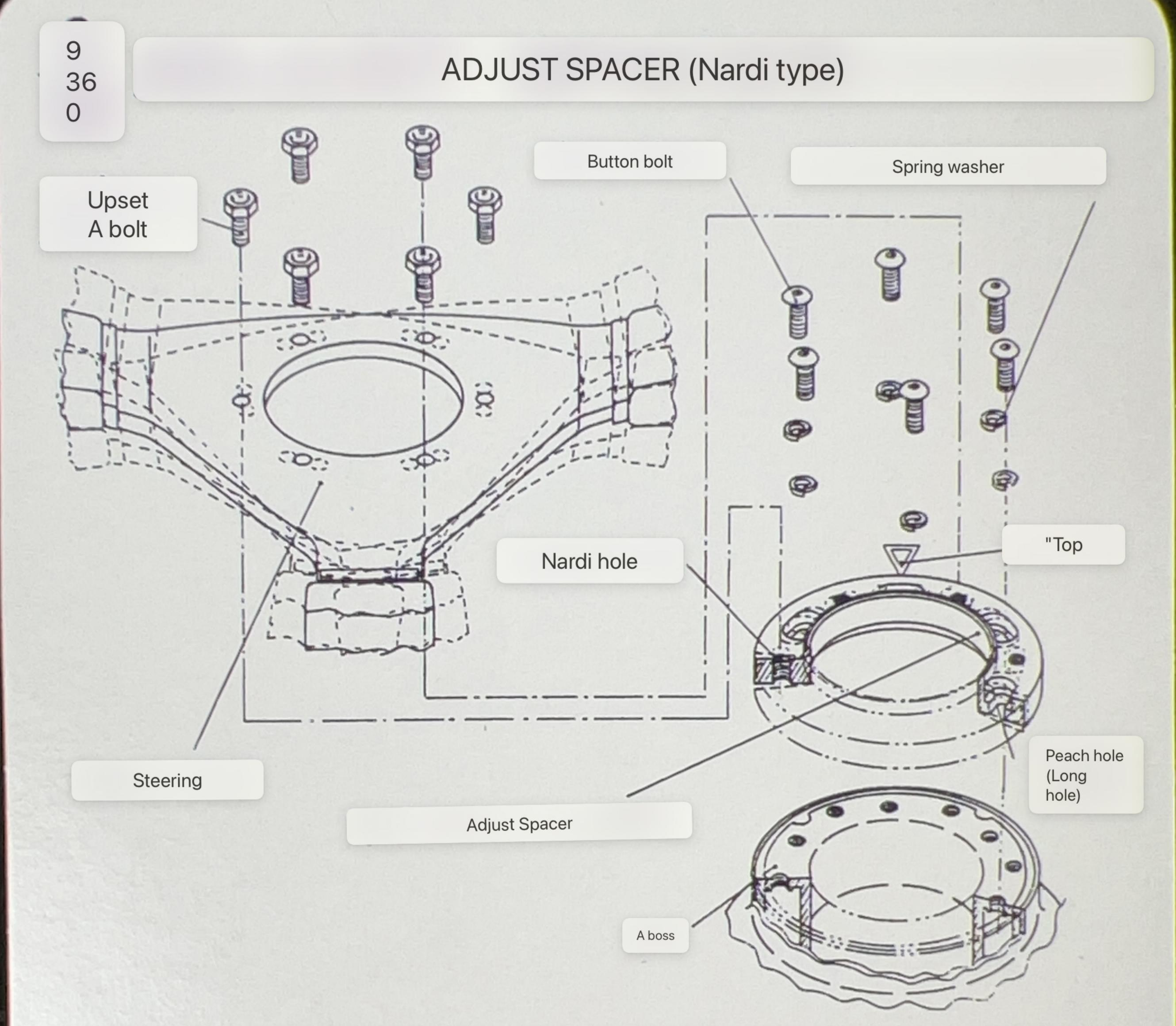
If you replace the genuine steering with a commercial steering wheel, if the steering direction does not straighten when it goes straight, please check the actual top position and remove the steering wheel. Next, adjust the center of the peach hole (long hole) of the adjust spacer to match the actual top position, and the button bolt Through the spring washer,
