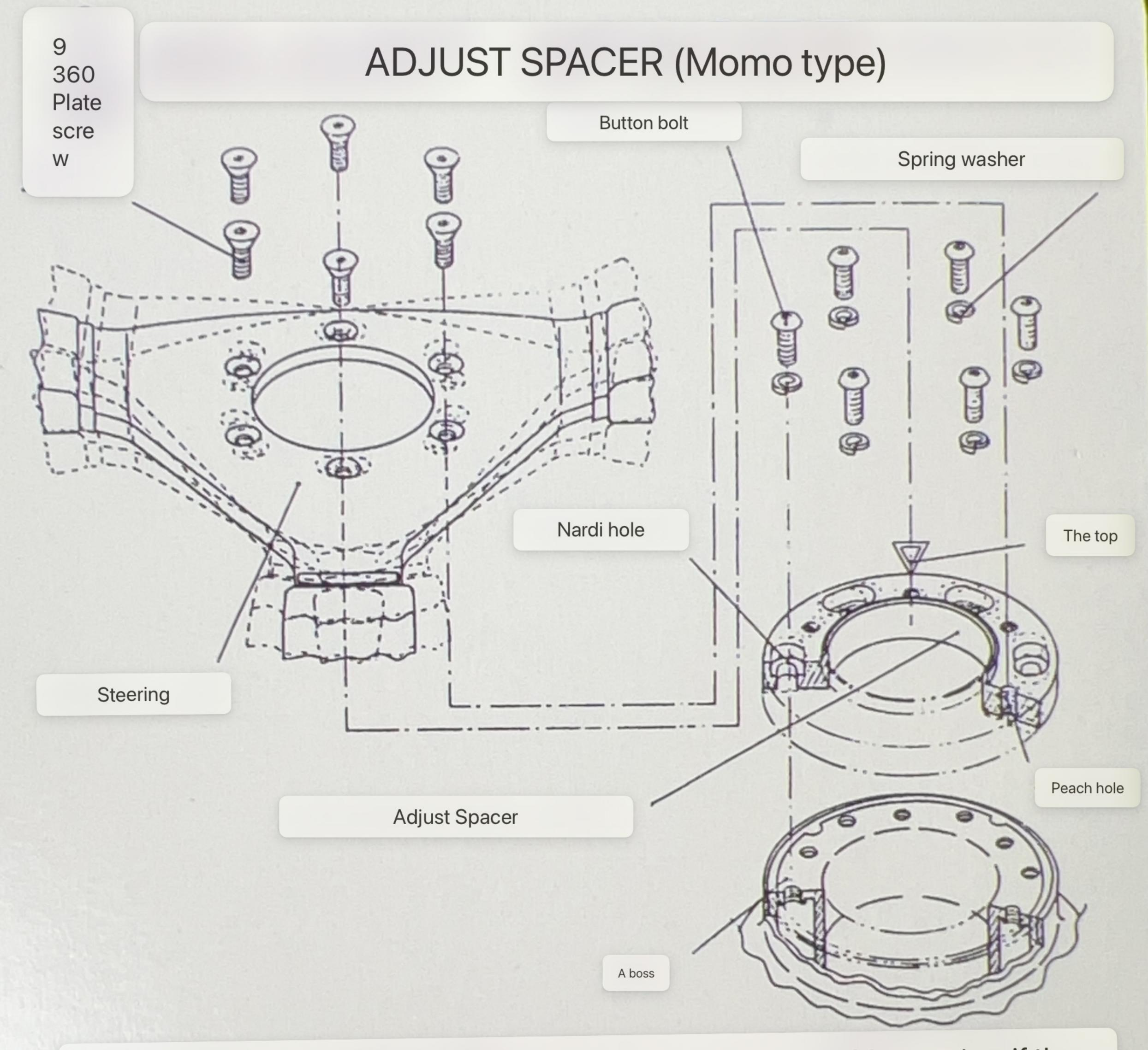
If you replace the genuine steering with a commercially available steering, if the steering direction does not straighten when going straight, check the actual top position and remove the steering wheel.
