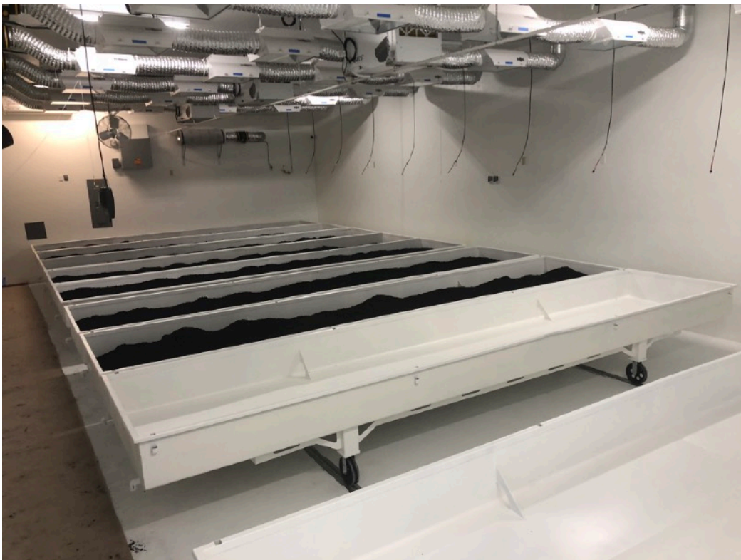
Rolling beds may be used to maximize space efficiency and energy output.
