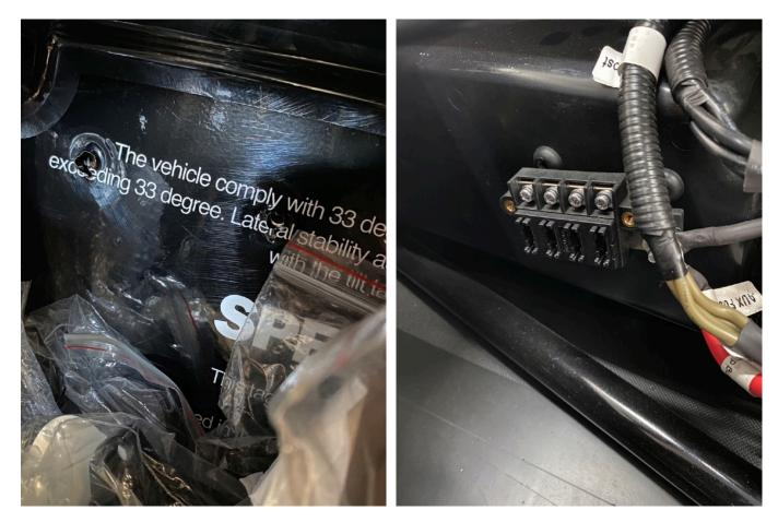
Reuse these allen heads to install the fuse block on our relocation plate.
