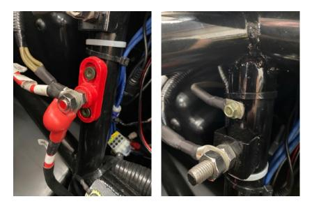
Reuse the 2 5 mm allens and 8 mm bolt to install the ground wire and relocation plate. Use the 6 mm hardware provided to mount the power post onto the relocation plate. Re-tighten the power post 16mm nut with positive cables.
