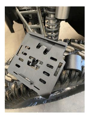
Use 14mm wrench. Position the tray on top of the roll bar as shown.
