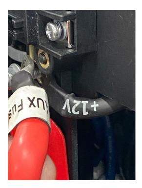
Reinstall the two positive wires to the fuse block. There is a black cable marked 12 V and a short red cable marked AUX Fuse. Shown above.
