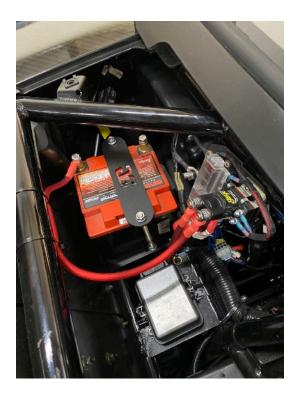
Connect the long battery cable to the left lug on the stinger solenoid and your new battery's positive cable to the right lug.
